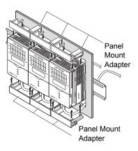
4. Install the long Mount Adapters on the two holes on the small Mount Adapter.
