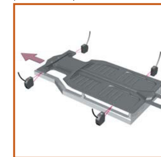
Measuring Car Body Widths (ZS-HLDS10)
