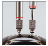
Since micropressure contact is achieved using the Actuator's own weight, these Sensor Heads are ideal for taking measurements where non-contact Sensors cannot be used, such as on transparent and glossy products or products that are easily scratched or warped
