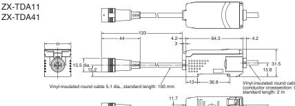
Vinyl-insulated round cable 5.2 dia. 10 conductors, (conductor crosssection: 0.09 mm², insulator diameter: 0.7-mm dia.), standard length: 2 m
