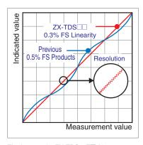
The long-stroke ZX-TDS04T $\square$  (4-mm measurement range) achieves high-precision measurement with the industry's top class of resolution (0.1  $\mu$ m) and linearity of 0.3 FS max.
